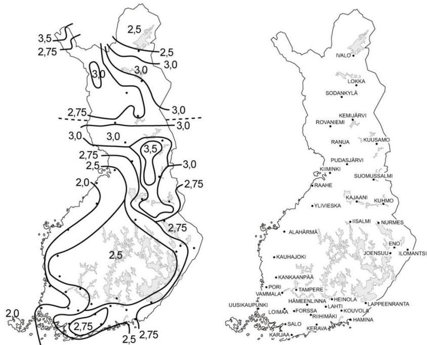
Figure 1. Characteristic values for snow load on the ground, in units of kN/m<sup>2</sup>. If the construction site is located in an area where the value is not constant, the intermediate values are obtained by linear interpolation in proportion to distances from the closest curves.
