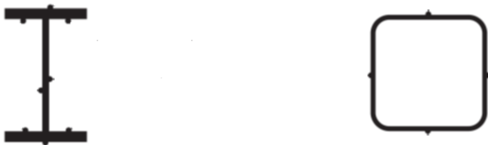
Figure 1. The dry film thickness measurement for fire protection paint is performed at the locations indicated in the figure
